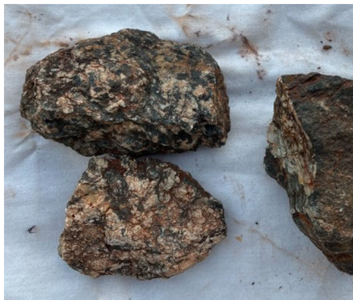
Photo 1: CGRC045–0.6g/t Au with elevated Ba(220 ppm),Cr(245 ppm),Mn(1,060 ppm),P(1,000ppm)and Sr(577ppm)
