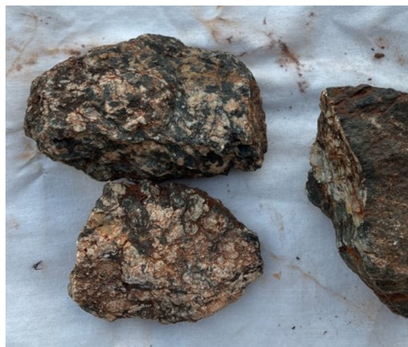
Photo 1: CGRC045—0.6g/t Au with elevated Ba(220ppm),Cr(245ppm),Mn(1,060ppm),P(1,000ppm)and Sr(577ppm)
