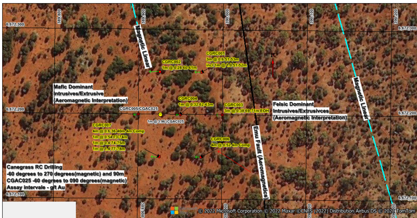
Figure 11: RC Drill Collars with significant gold intersections
