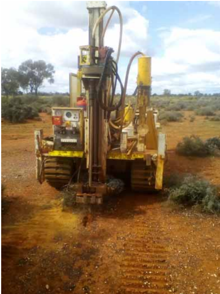
Vacuum Drill Rig in Operation and the Low Impact Nature of the Drilling
