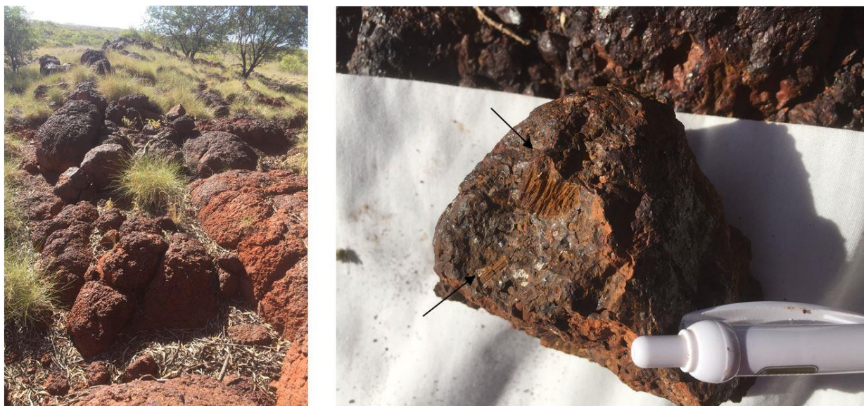
Figure 5: Channel Iron Deposit (CID) outcrop at left showing a close up of the pisolitic iron mineralisation at right with arrows showing wood fragments (brown) typical of CID iron mineralisation.
